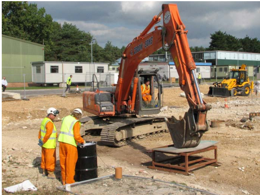
Figure 6: Bucket Monitoring of Soils using Table & Sodium Iodide Detector
