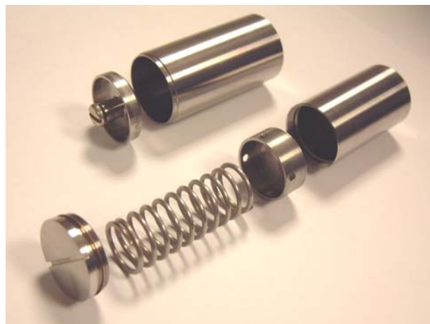
Fig. 2. The AE4043/n source component configuration minus the spring locators
