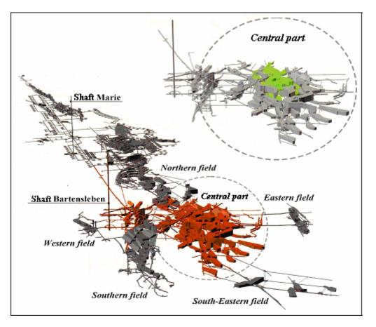
Fig. 1 Mine openings and cavities of the central part to be backfilled in advance (green)
