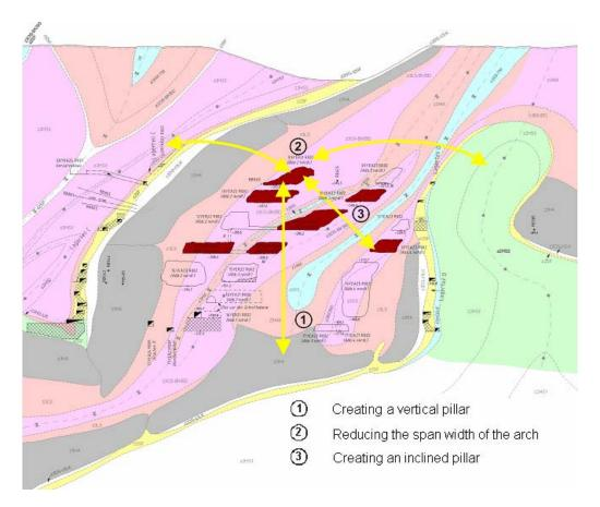
Fig. 2 System of arches and pillars due to stabilization measures.
