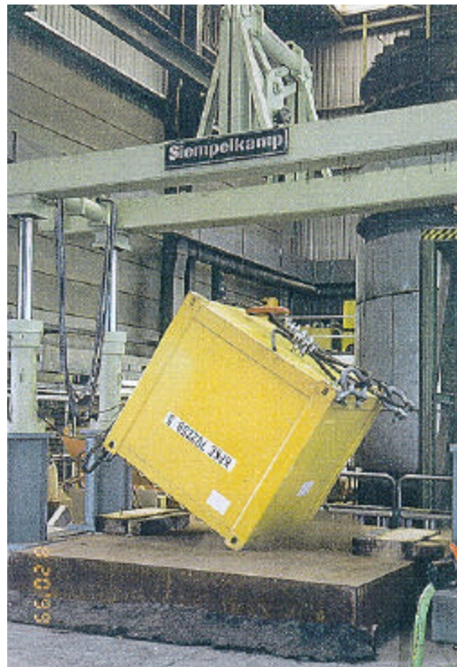
Fig. 7: 0.8 m drop test
