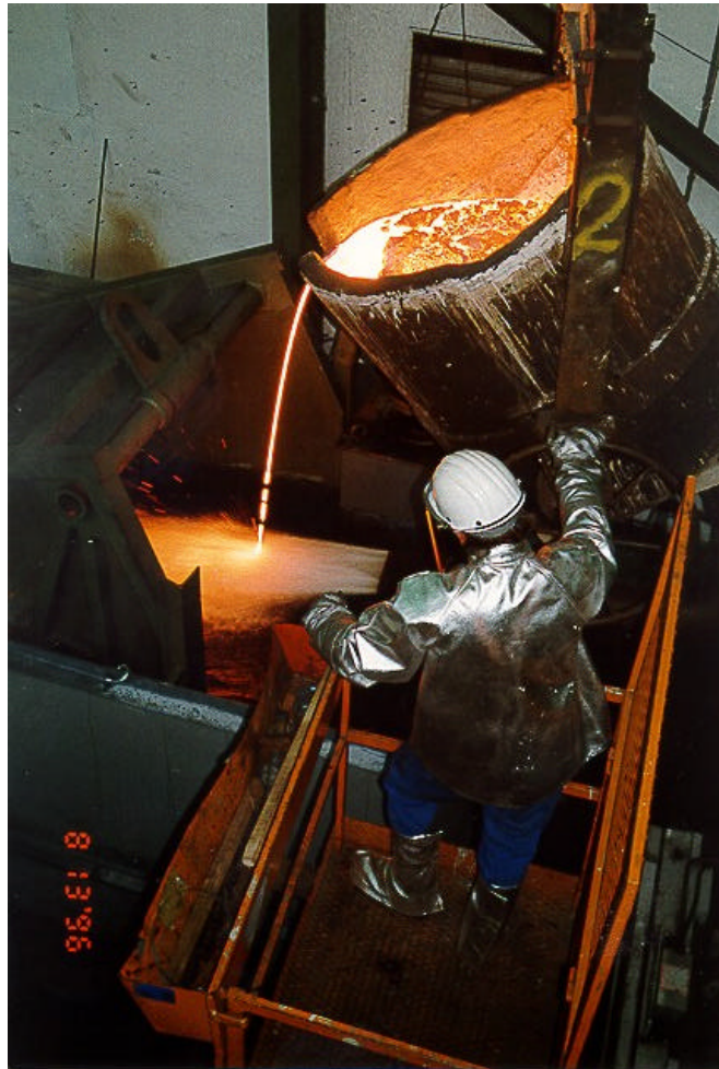
Fig. 3: Granules production in Siempelkamp's CARLA plant
