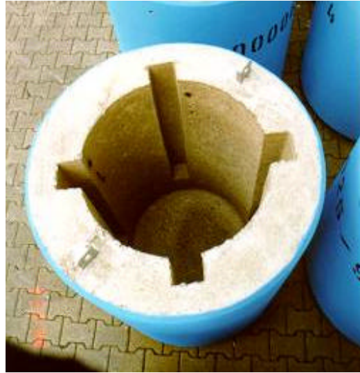
Fig. 5: View into a granule concrete shielding container for 200 l drums
