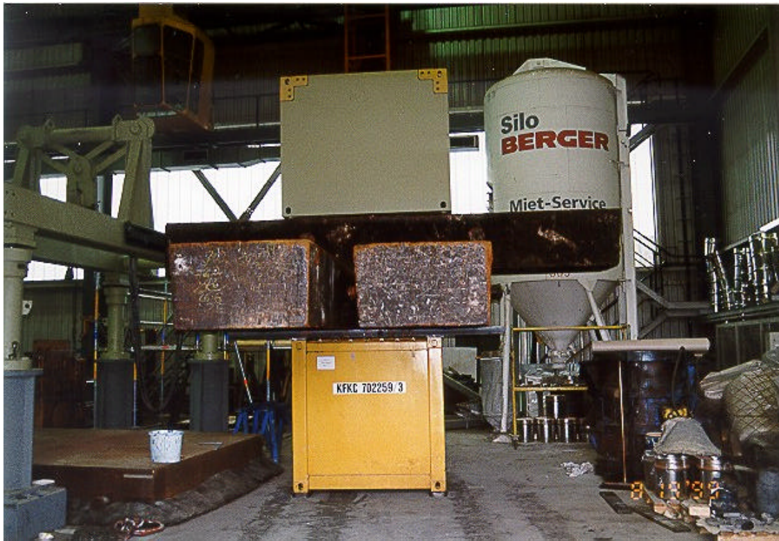
Fig. 8: Stackability test for PSC-container
