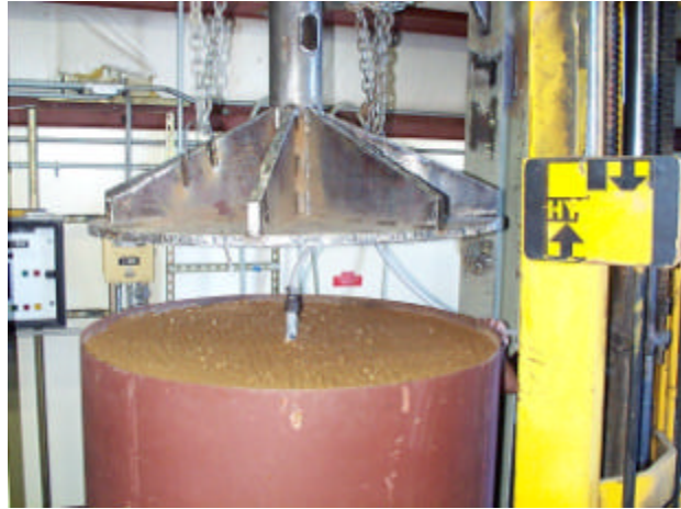
Fig. 4. Placement of load cell plate on the 1.22-meter sand tank.
