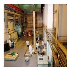
Figure 1: Recovery of Floor Storage Liners Using Overhead Crane
